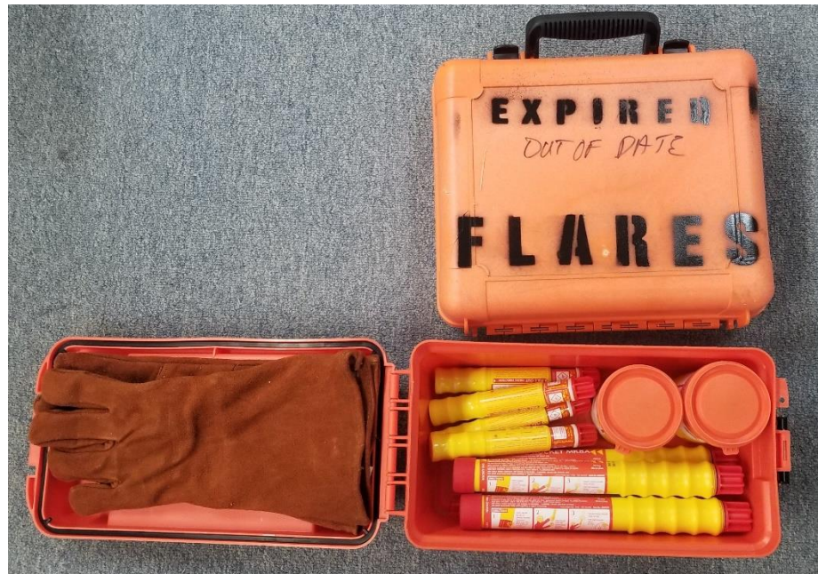
Figure 3 Watertight flare storage box with welding gloves and our recommended 4 SOLAS rocket parachute flares, 4 SOLAS handheld flares, and two SOLAS smokes. A container for expired flares is also shown.
